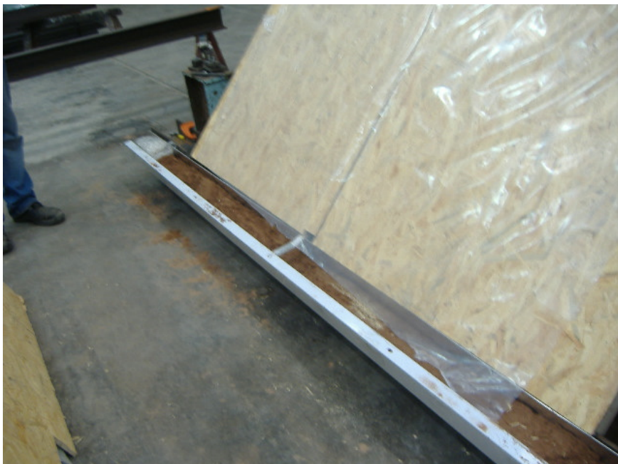
Plate 4 - Impact Test Set-up Showing Gutter Half Filled with Sand
