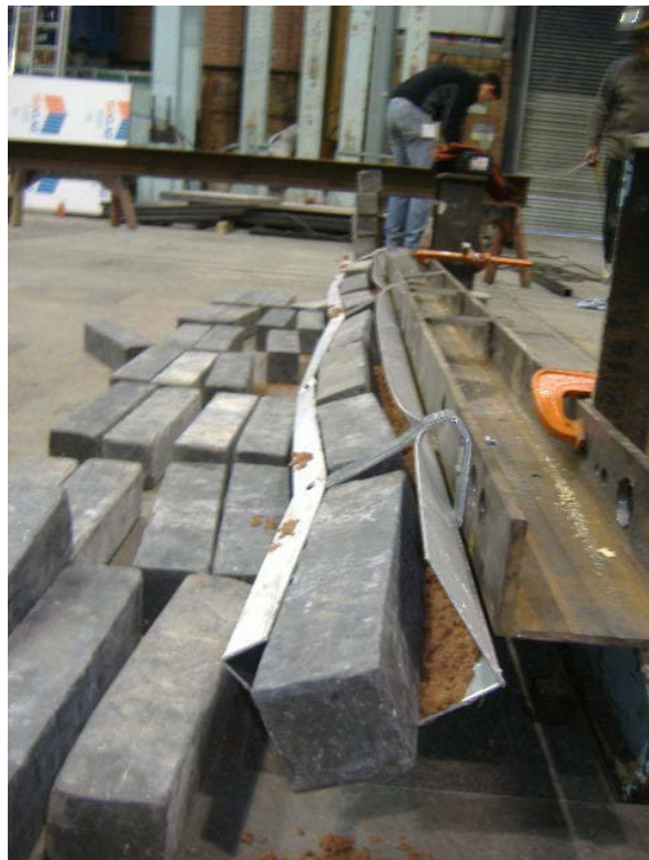
Plate 2 - Showing Bending of Brackets at Failure
