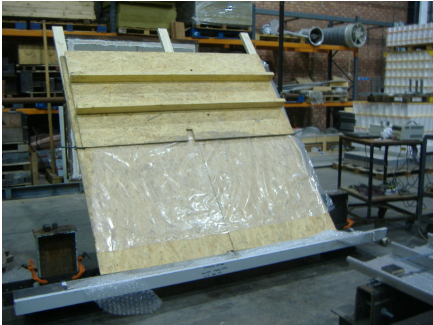
Plate 3 - Impact Test Set-up
